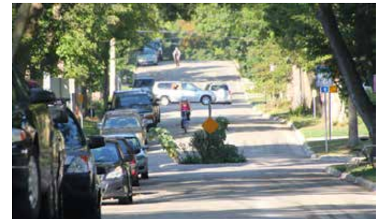
Mini traffic circles may be used to lower motor vehicle speeds near intersections with bike boulevards. Image: NACTO
