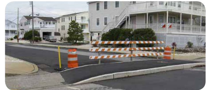
This permanent roadway closure in Ocean City, NJ preserves bicycle and pedestrian access. Image: The RBA Group
