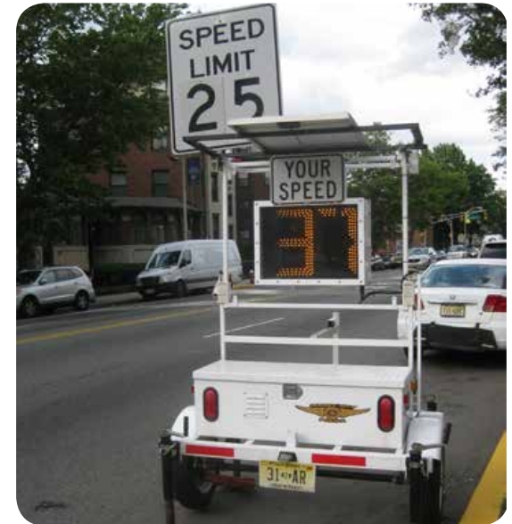
Temporary speed feedback trailer in Jersey City, NJ. Image: The RBA Group
