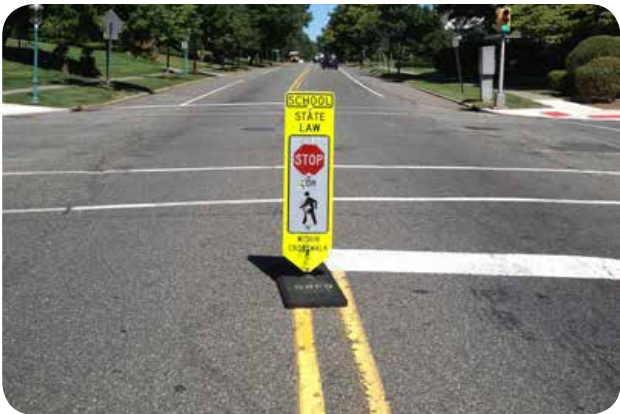
In-Street Stop for Pedestrians Sign with SCHOOL plaque mounted above the sign in Glen Ridge, NJ. Image: The RBA Group
