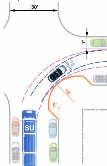
Single Unit (SU) Truck Turning Radii vs. Personal Car Turning Radii. Image: The RBA Group
