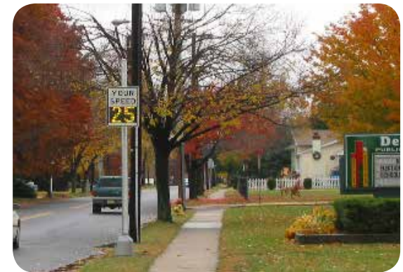
Permanent speed feedback sign in front of an elementary school in Delanco, NJ. Image: NJDOT
