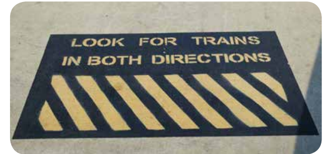
Example of a clear, concise warning message communicated by this pavement marking. Image: FRA, Guidance on Pedestrian Safety at or Near Passenger Stations
